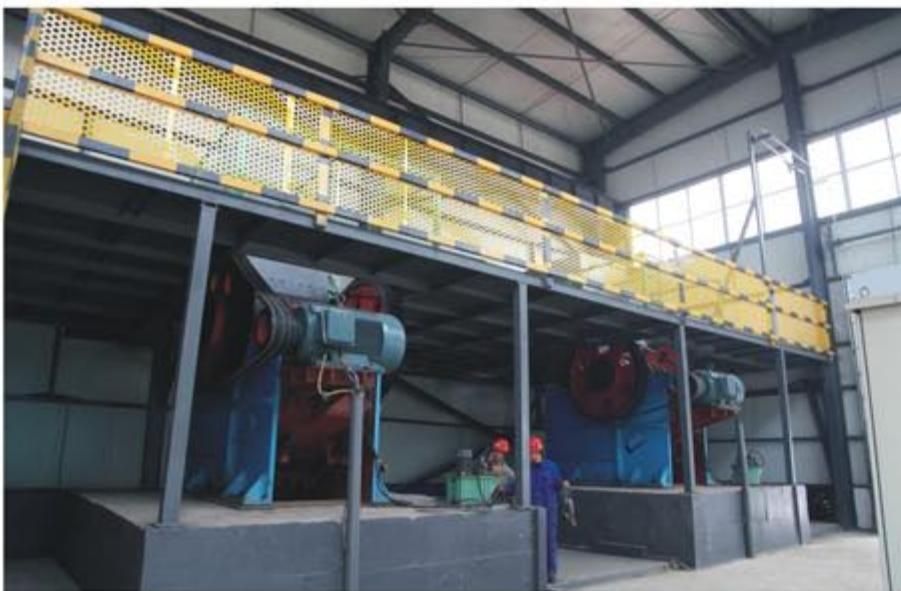
Jaw Crusher is widely used for rough and secondary crushing on metallurgy, mining, construction, chemical and cement etc. According to structural character, there are single toggle type (crank rocker structure with the movable jaw doing intricate movement) and double toggle type (crank rocker structure with the movable jaw doing simple movement).
